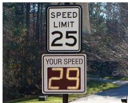
Figure 3. Sample of Radar Feedback Signs
